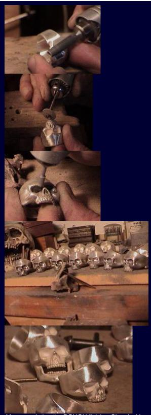
After completing the ROUGH finish a Chemical is used to Stain the Silver BLACK in the Desired areas like the Eye-Sockets, nose and between the teeth.
