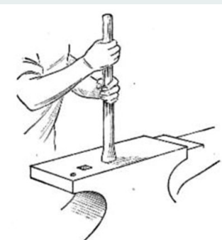
Fig. 15. Upsetting by Ramming
