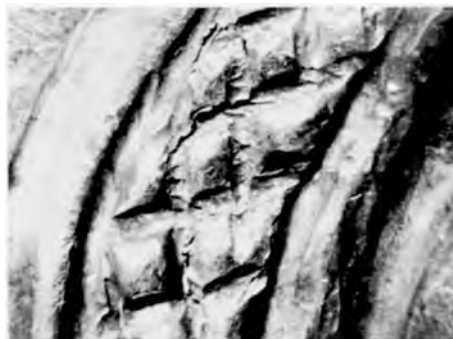
1.4 Horse rhyton. The "toothed" surface has failed to bond the foil to the silver. Photo by Katharine C. Ruhl.
