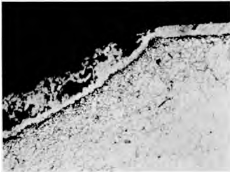
1.26 Torso insert, section through a decorative punched hole. Accumula- tion of spongy gold is seen within depression. Magnification 300X. etched by K_2Cr_2O_7 + NaCl + H_2SO_4 , diluted 1:9.
