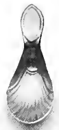
Caddy Spoon, struck in a die from fused-plated sheet metal, by T. Law & Co. Date 1785. Author.
