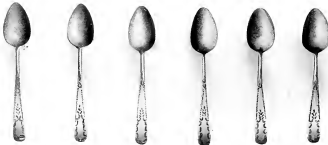
Tea Spoons, shanks made from plated drawn wire, and chased by hand, the bowls struck from a die and soldered on separately, by T. Law & Co. Date 1777. Author.
