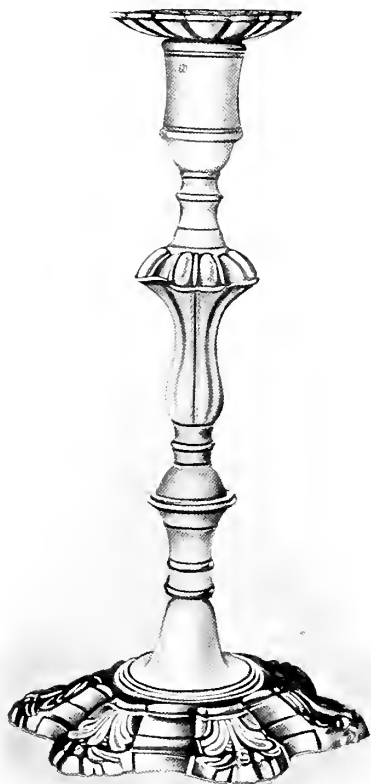
Sheffield Plate, 10 in. shell pattern Candlestick. The collettes and neck, also capital, are roughly swaged. The shoulder mounts, foot and nozzle have been struck in cast steel dies, and afterwards chased by hand. Up the stem will be noticed a little chasing to take the eye off the soldered seam, JH marked on the capital. Probably by Joseph Hancock. Date 1755—1760. Author.
