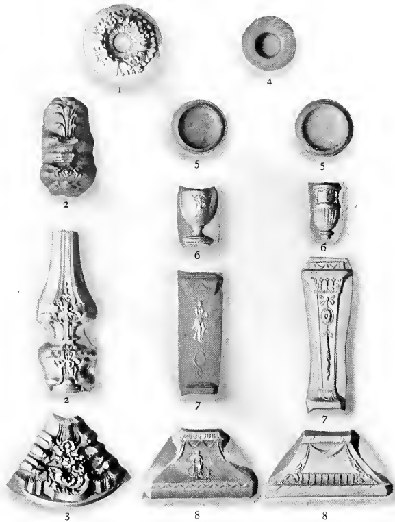
Stampings from Dies showing the various parts used in the construction of Candlesticks.
