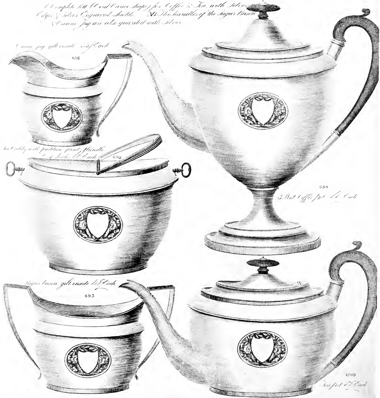
Illustrated Design from Catalogue, about 1795. An early example of a combined Coffee Service, with Caddy. The first illustration showing the separately soldered-in shields for engraving.
