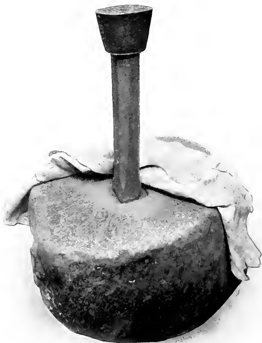
Hammering Stake 2 ft. 3 in. high, in use for over 100 years. On the wooden base will be noticed marks caused by countless numbers of small nails that have from time to time been driven in for fastening down a leather sheet to intercept any dust that might arise
