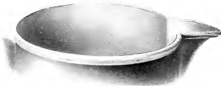
Jug, showing method of protecting top and lip with a plated drawn wire mount. Date 1783.
