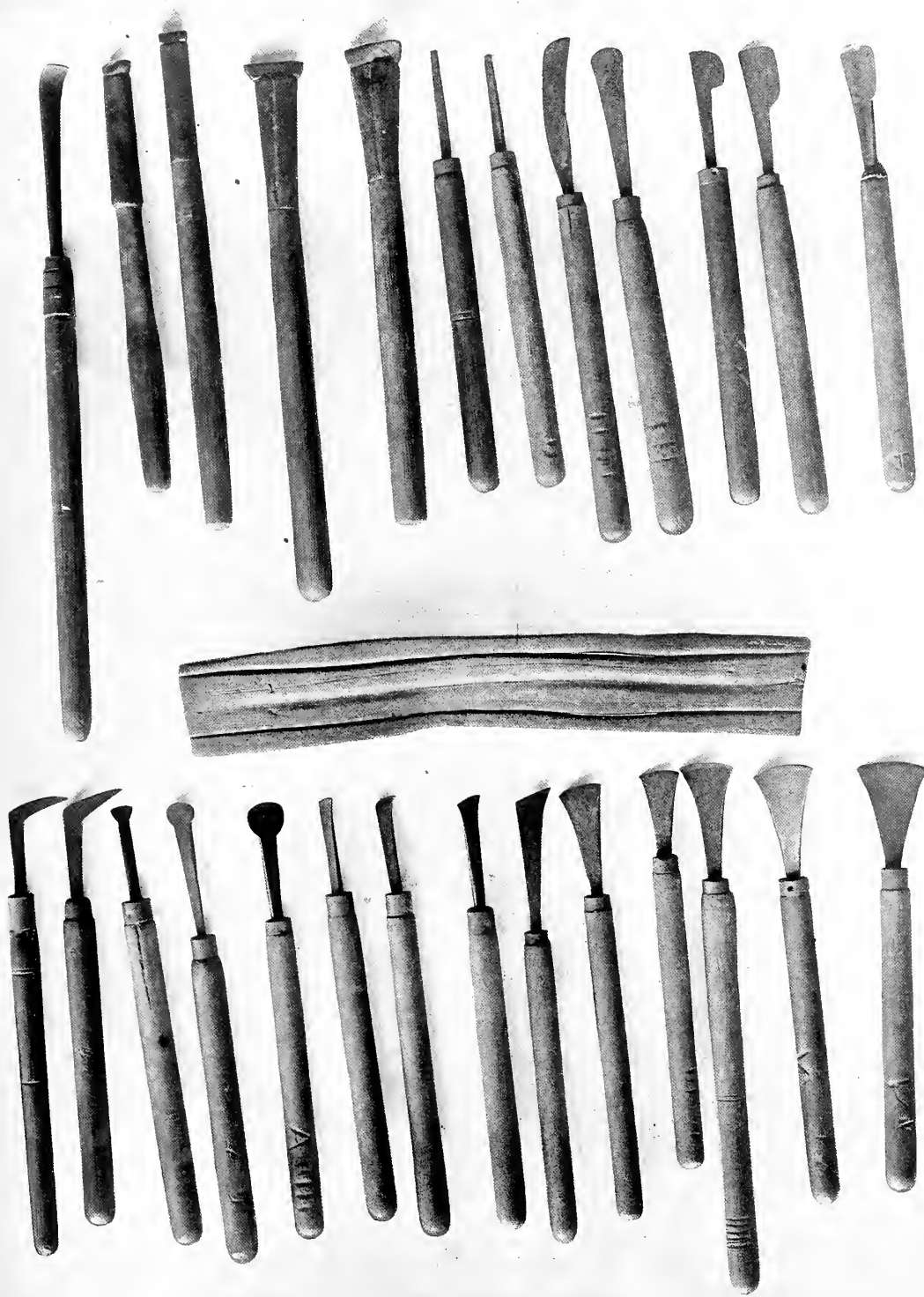
Illustrations of Burnishing Tools, showing the leather strop on which the burnish is constantly rubbed during the process. The marks on the handles are made by the various owners of the articles.
