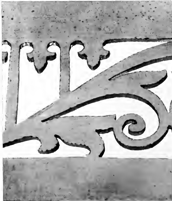
Enlarged Section of Fused Plate, showing the result of saw piercing. The jagged edges raised by the saw are clearly discernible.
