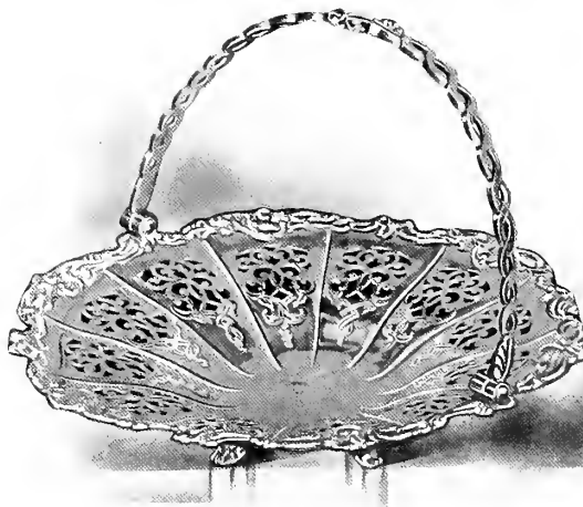
Card Tray, handle and body of "argentine" metal (see page 137). The mounts of silver (filled), body hand saw pierced and flat chased (electro-plated), by T. Bradbury & Sons. Date 1848. Miss Bradbury, Sheffield.
