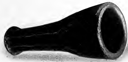
Drafting Punch, 8\frac{3}{4} in. long, 4 in. across mouth, being used by the stamper in forefront of illustration on next page.
