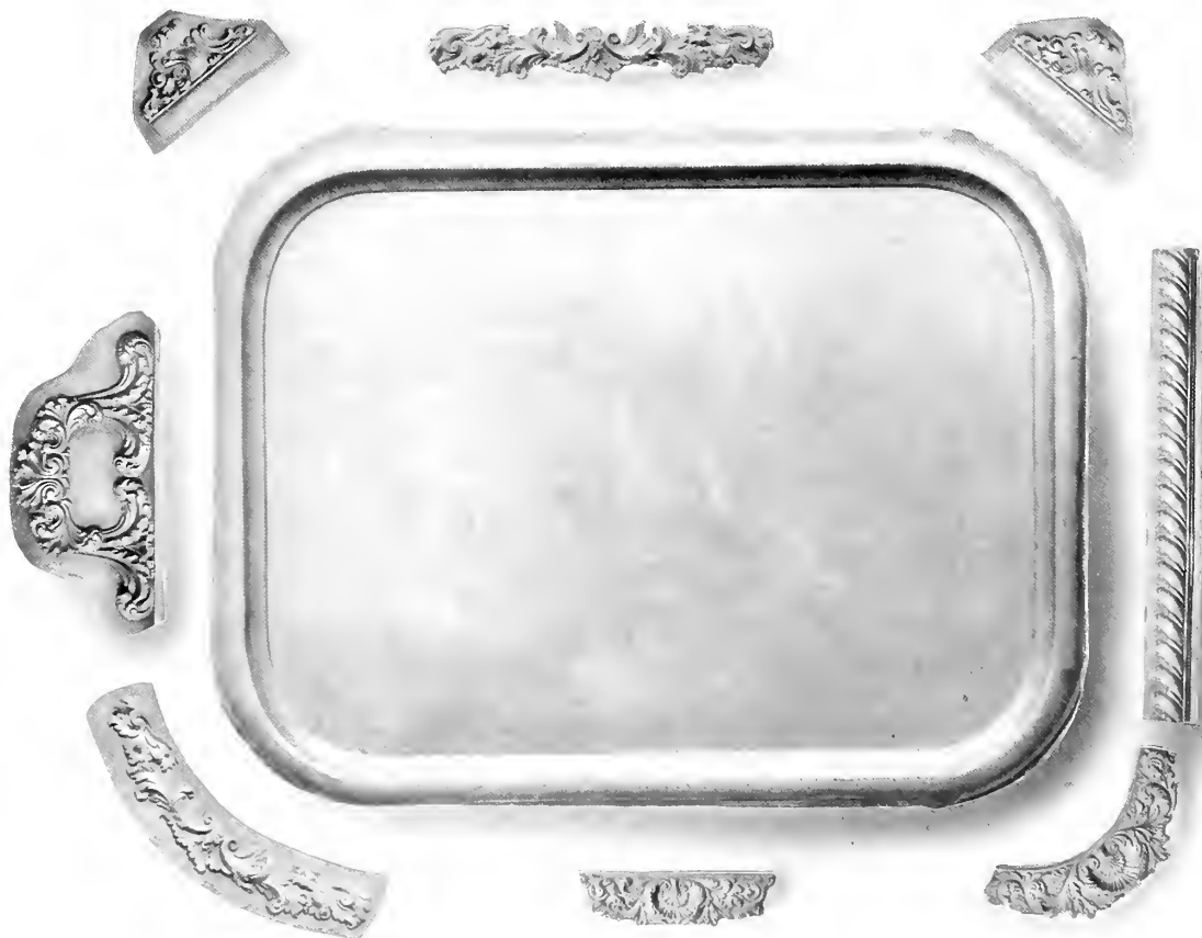
24 in. Tray Plate after being stamped and swaged, also showing various sections of silver mounts for handles, feet and borders as they have left the dies. Section of florid mount on top shows the mount filled and filed preparatory to soldering it to the border of Tray.
