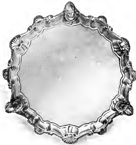
Reverse of 8 in. chased Salver. The under side of swage being of thick metal and for the purpose only of giving strength, has not been struck home in die, as is the case with the front side, which is stamped from metal of a much thinner gauge.
