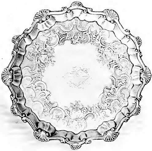
8 in. Salver, with chased front. Made from two sheets of single side plated metal, soldered back to back and secured between the edges of the swage and mount—also in duplicate. In this instance the mount and swage are conjointly cut in the same die, a method abandoned after the introduction of silver mounts. Probably made before the invention of double side plating.
