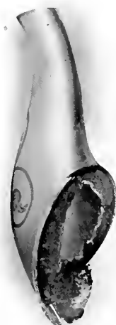
Teapot Spout, made of German silver, electro-plated. This has dropped off after 30 years' wear owing to decomposition referred to by Mr. A. S. Johnstone (see Page 139). The illustration is also instructive as showing how the tannin in the teapot spout will accumulate until finally it entirely chokes up the passage.
