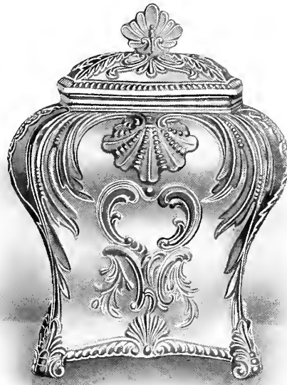
Sheffield plated specimen Caddy, some 15 years later than that made by Paul Lamerie, executed entirely by the aid of dies. It will be noted how greatly the shape of the caddy is improved by the aid of the die. Being more graceful in outline it is also much sharper in definition.
